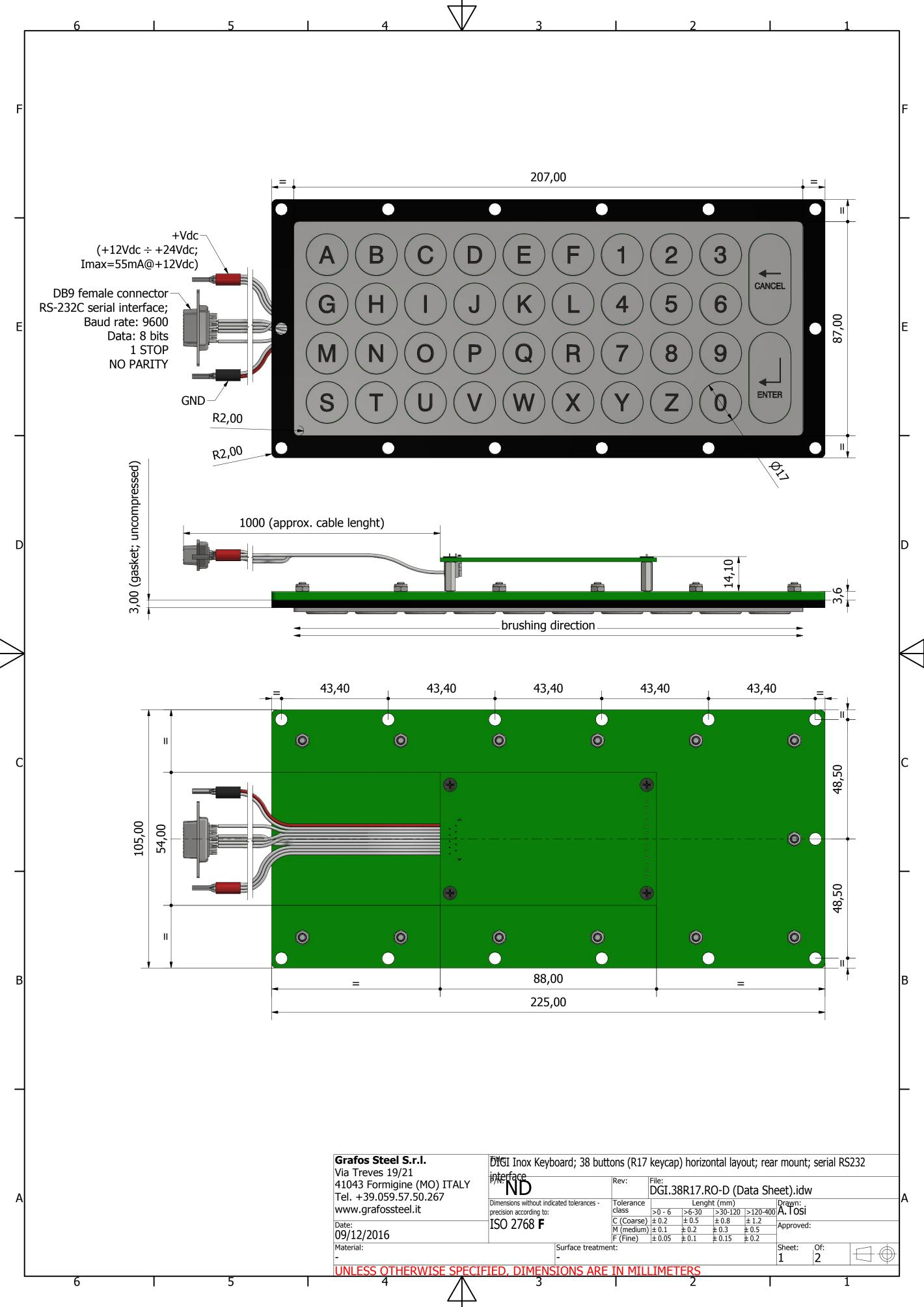
AISI316L Stainless steel buttons; symbols: chemical etching + color infill AISI316L Stainless steel front panel (2 mm thick) EPDM rubber sealing gasket-3 mm thick (uncompressed)
